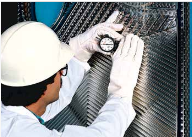
Draw depths of plate chevrons are meticulously monitored.
