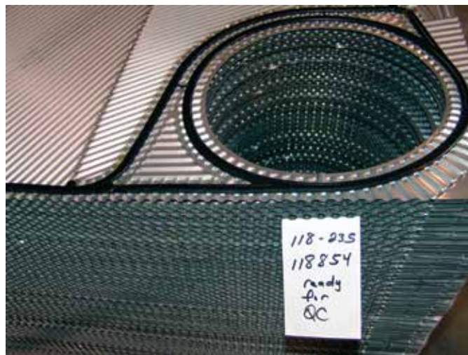
Plates are pressed in virtually any cold-formable metal and furnished with the right gasket materials to match your process conditions.
