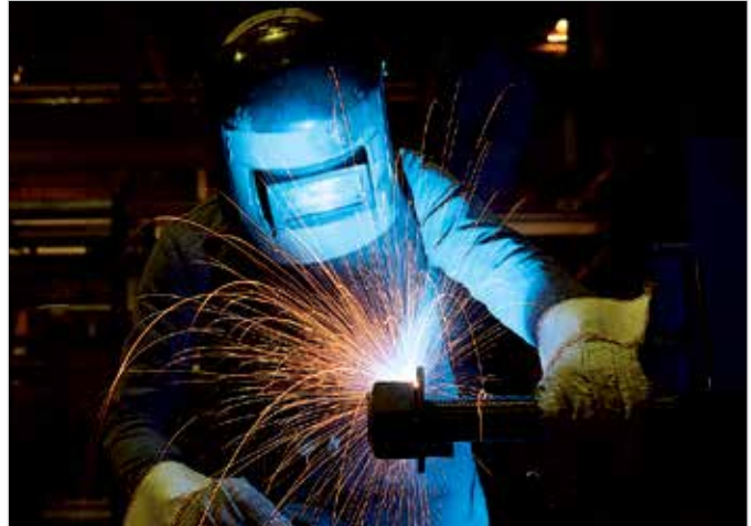
GTAW and GMAW welding processes are utilized on nozzles and end frame reinforcing bars, respectively.
