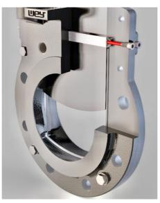
The transverse seal can be repacked at any time and under full pressure using the lateral packing screws.
