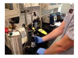
The c-DGM is a versatile tool for checking dissolved  $\mathrm{CO_2}$  and  $\mathrm{O_2}$  content throughout the process. The ISD is a robust instrument for sampling without air intake and is particularly suitable for determining the DO and  $\mathrm{CO_2}$  content when used in with the c-DGM.
