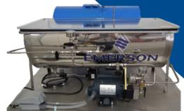
The pressure reducing valve, spray water valve, and spray nozzle all play an equally important role in maintaining adequate temperature control. The desuperheater nozzle is physically the smallest component of the system, but it is vital to the success of the desuperheater station.
