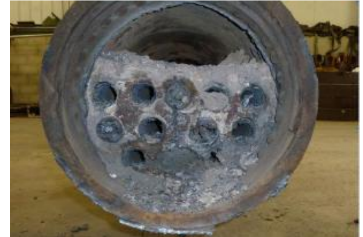
Solid Scale Around Boiler Tubes Source: Discover Live Steam
