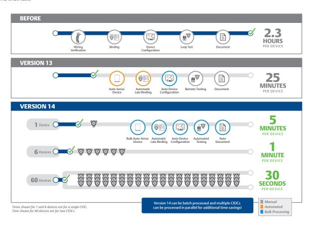
I/O Studio allows you to configure IO devices even before the device location is known, commissioning policies and loop test settings that will be used by the DeltaV Device Commissioner. I/O Studio will completely decouple hardware and software configuration and development, and enable easy, one-click commissioning via the DeltaV Device Commissioner.
